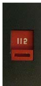
Voltage selector switch set to 115V
